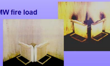
Fire load before and after fire test
