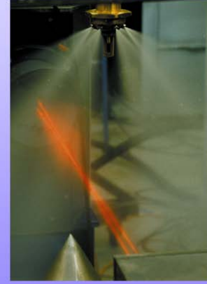
Droplet measurement with laser - doppler equipment
