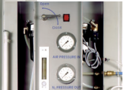
Compressed air regulation
